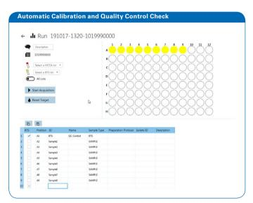
◆ The MALDI Biotyper System can automatically be checked by analysing Bruker Bacterial Test Standard (BTS) before each run. Using BTS for the quality control of the MALDI Biotyper assures the highest data reliability and measurement reproducibility.
